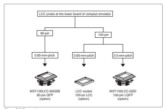
Figure 2.9 Connecting target system
